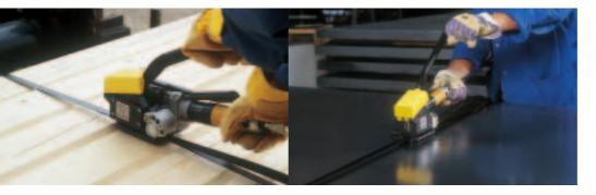
Applications The ideal tool for applications where the tool cannot be suspended and where a high performance within a wide range is required. Very popular strapping tool in the lumber- and metal industries.
