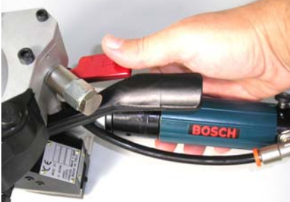
PHASE 2; SEALING AND CUTTING THE STRAP
