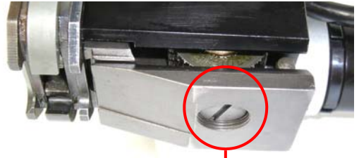
TURN THIS TO ADJUST THE GAP BETWEEN THE FEEDWHEEL AND THE PRESSURE BUTTON
