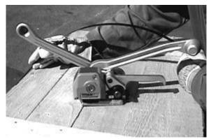
Pull through the strap end until is in the center of the package beneath the upper run of strap and juts out approx. 15 cm.
