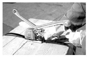
5. The right hand grasps the tension lever 508 and moves it back and forth to obtain the desired strap tension. At the same time the left hand holds the cutting lever 35.
