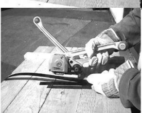
3. With the left hand hold the upper and lower run of the strap together. Both straps must be placed exactly on top of one another. Grip and press rocker 509 together with the cutting lever 35 with the right hand. Insert the steel strap laterally until it strikes against the case wall, ensuring that the lower run of strap projects slightly out of the tool at the front. The right hand now releases the levers which have been pressed together.
