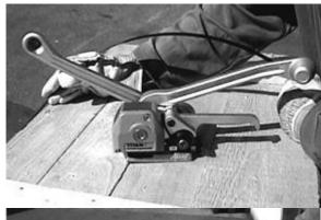
2. Pull through the strap end until it is in the centre of the package beneath the upper run of strap and juts out approx. 15 cm.
