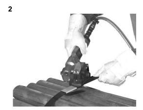
Position the pneumatic sealing tongs (DPZ-L) on the sealing sleeve (as shown in the photo) and notch the sealing sleeve by the actuation of the joining lever. At the same time the joining lever snaps in automatically. Releasing is done automatically after the notching of the seal and of the steel strap have been completed. Interruption of the joining process is possible at any time by pushing the STOP key.
