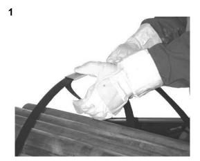
Take the jack (PR 33) in your right hand and open it by pressing the lever. Then slip it on the steel strap from the right to the left acc. to the photo. Release the lever and tension the steel strap by turning the turning valve to the left. The tension of the strap desired (max. 6 bar) is achieved by the control of the air pressure on the pressure gauge of the maintenance unit.
